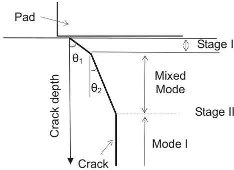
Fig. 2. Schematic view of fretting crack propagation.
