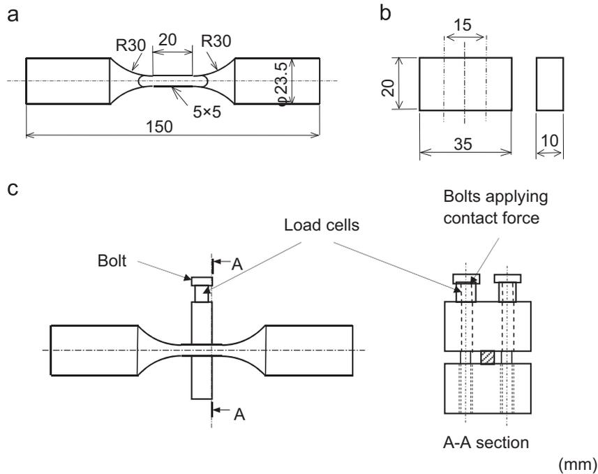
Fig. 3. Shapes of specimens and test apparatus: (a) specimen, (b) contact pad, and (c) test apparatus.
