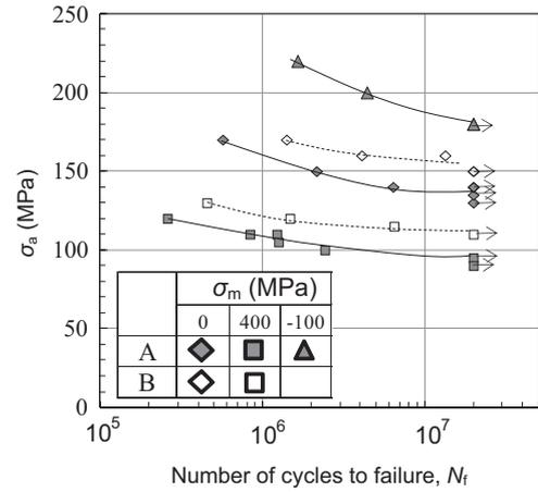
Fig. 4. S-N diagram of fretting fatigue tests.
