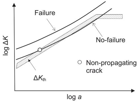
Fig. 1. Schematic of small-crack propagation model at fretting fatigue.
