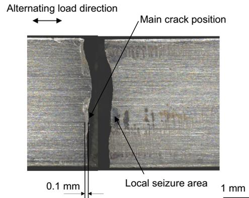
Fig. 5. Side view near contact edge of failure specimen. (Sample A:  $\sigma_m=0$  MPa,  $\sigma_a=150$  MPa).
