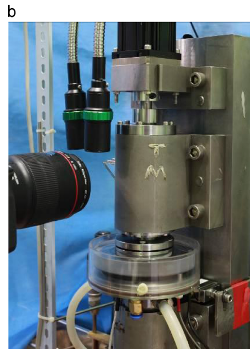
Fig. 1. (a) Schematic diagram and (b) photograph of the test rig used to examine the two-phase mechanical face seals with LST.
