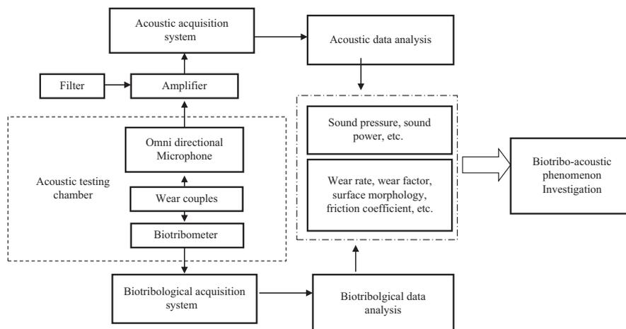
Fig. 1. Schematic of the biotribo-acoustic testing flow chart.
