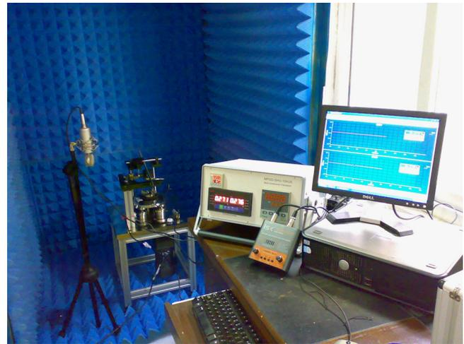
Fig. 2. Biotribo-acoustic testing system for orthopaedic biomaterials.
