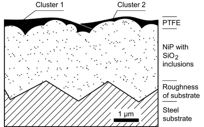
Fig. 2. Schematic representation of NiP coating with SiO<sub>2</sub> and PTFE (cross section).
