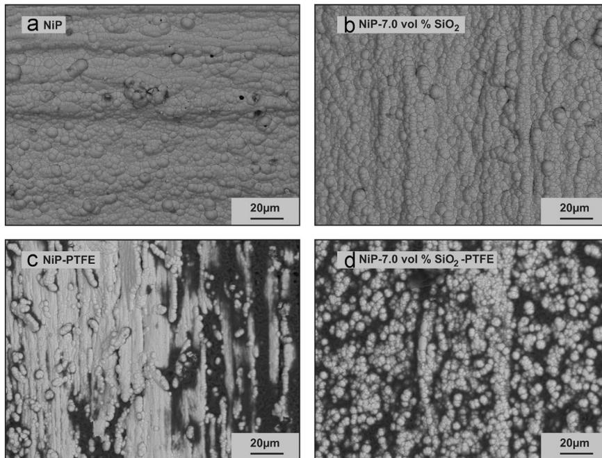
Fig. 1. SEM images of surfaces of as-deposited coatings.
