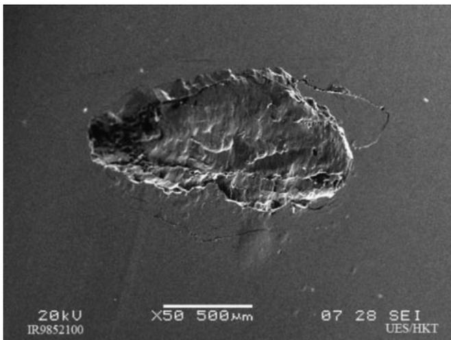
Fig. 1. Typical fatigue spall in AISI 52100 (from [4]).
