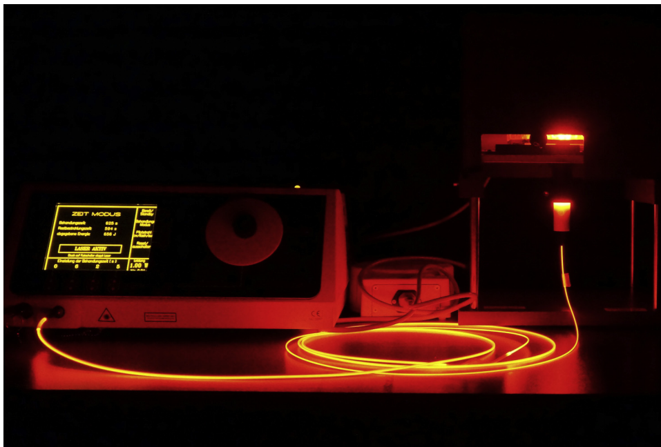
Fig. 2. Irradiation setup during PDT: Laser (left), fibreglass probe (middle), 96-well plate in the irradiation chamber (right).
