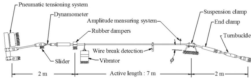
Fig. 1. Resonance fatigue test bench.
