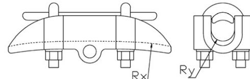
Fig. 2. Radii  $R_x$  and  $R_y$  of suspension clamps.
