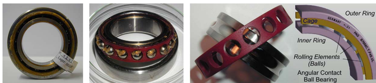
Fig. 1. Tested bearing (left) and disassembled test-bearing (middle-left) with the main components: the inner and outer ring, the rolling elements (balls: \varnothing=7.93\text{ mm} ) and the laminated fabric cage. Cage and inner ring of an untested reference bearing (middle-right), schematic cross-section of the angular contact ball bearings used for the tribological tests (right).
