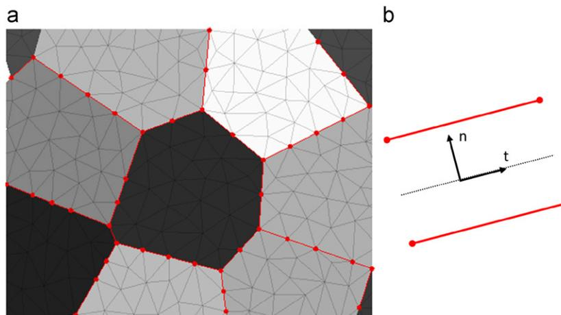
Fig. 2. (a) Finite element and cohesive zone element mesh of the material microstructure and (b) local coordinate system of the cohesive zone element.
