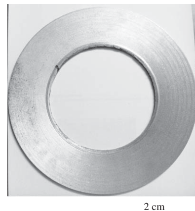
Fig. 1. Photograph of as-machined A359–20 vol% SiC composite disc.
