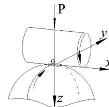
Fig. 2. Ball-cylinder model.
