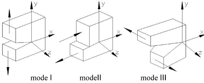
Fig. 1. Mode of crack surface displacement.
