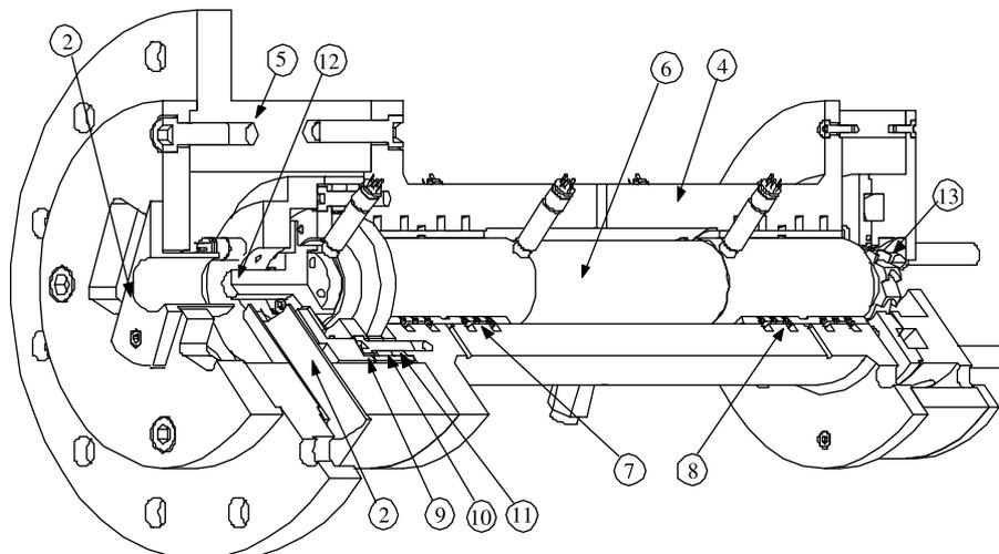
Fig. 2. Section of the spindle and the load devices.
