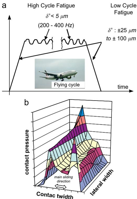
Fig. 2. (a) Illustration of the complex loading sequence imposed during a flying cycle; (b) illustration of the complex pressure field distribution in the blade/disk contact.
