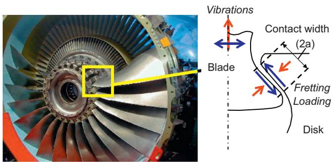
Fig. 1. Illustration of fretting loadings in the turbo engine blade/disk interface.
