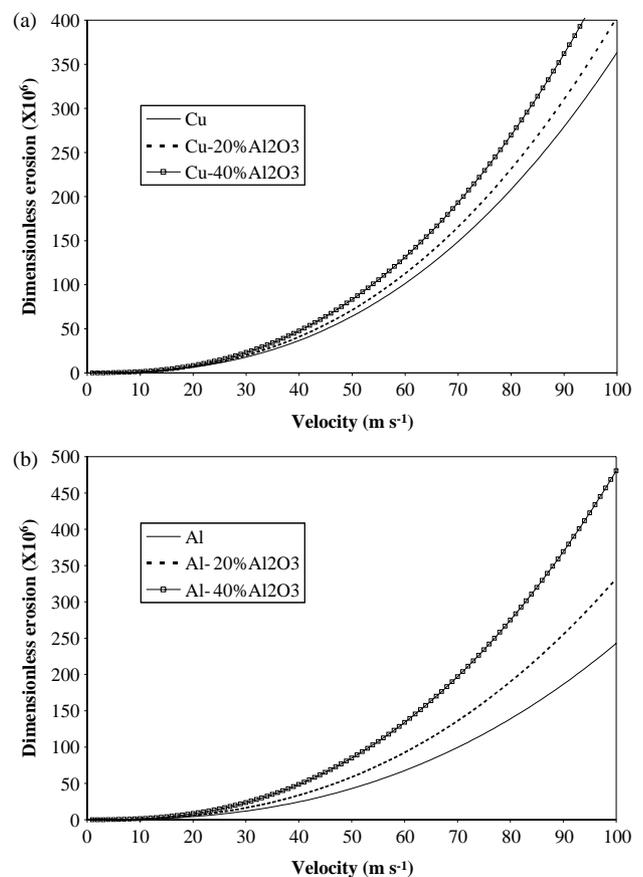
Fig. 2. Dimensionless erosion prediction of (a) Cu/Al<sub>2</sub>O<sub>3</sub>, (b) Al/Al<sub>2</sub>O<sub>3</sub> MMCs.
