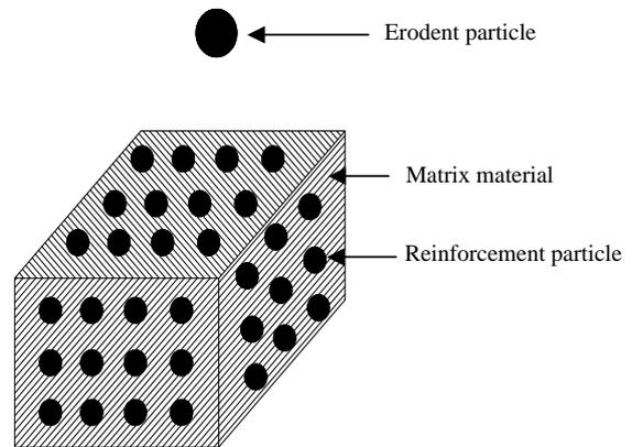
Fig. 1. Schematic diagram of an erosion event for a particulate reinforced MMC.
