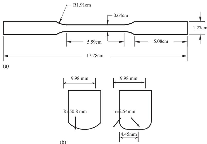
Fig. 1. Schematics of (a) specimen and (b) pad.
