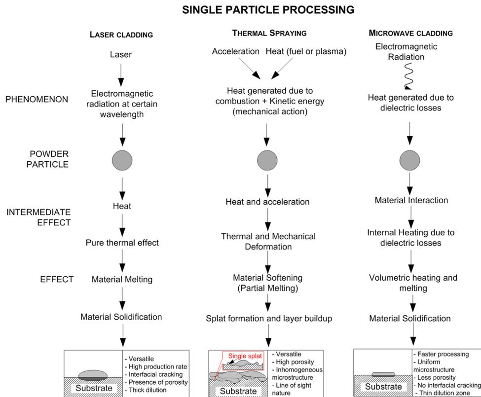
Fig. 1. Schematic diagram illustrating single particle processing.
