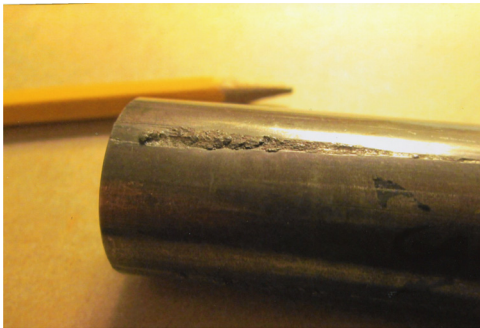
Fig. 1. Cylinder that galled on removal from a conforming cylinder.
