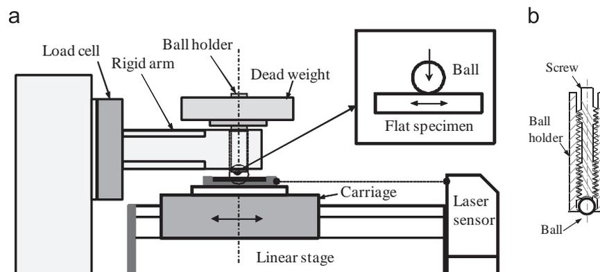
**Fig. 1.** Schematic illustration of the apparatus for reciprocal sliding testing: (a) testing machine, and (b) a ball holder with a screw.
