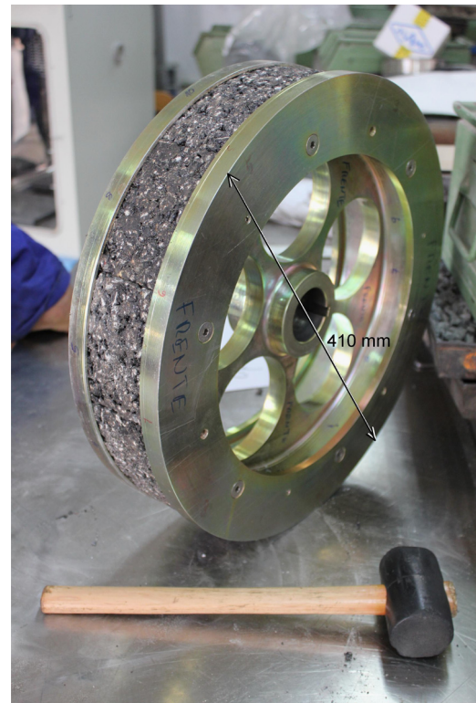
Fig. 2. New road wheel with specimens of the bituminous mixture.
