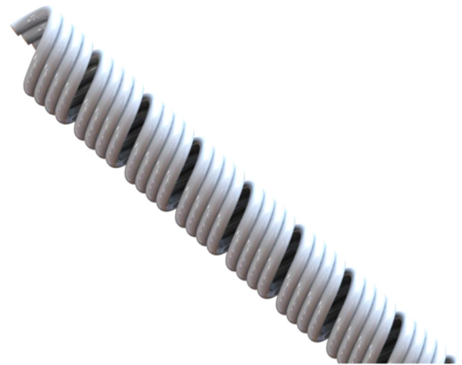
Fig. 2. Nickel alloy tribopartner for the implementation of the U-bend test.
