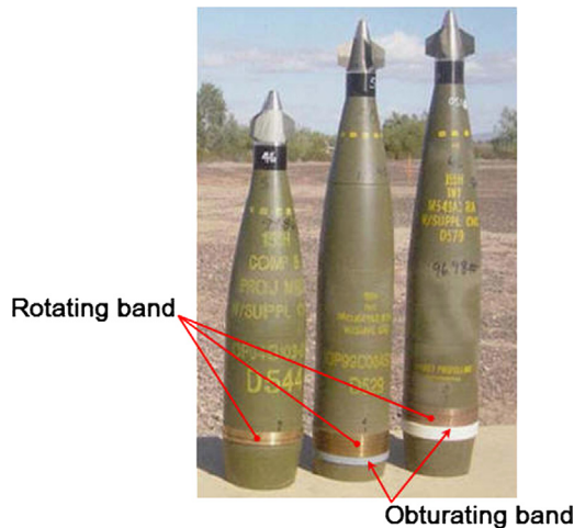
Fig. 2. Projectiles with rotating band and/or obturating band.
