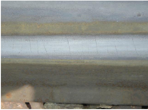
Fig. 1. A crossing nose with RCF cracks. With longitudinal slip, they are perpendicular to the running direction of the wheel.
