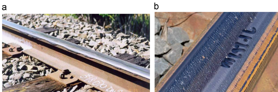
Fig. 1. (a) Typical rail plastic flow [11] and (b) rolling contact fatigue profiles of a rail in service [12].
