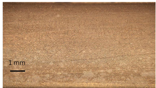
Fig. 2. Bore surface of Barrel 1 at 450 mm from the RFT.
