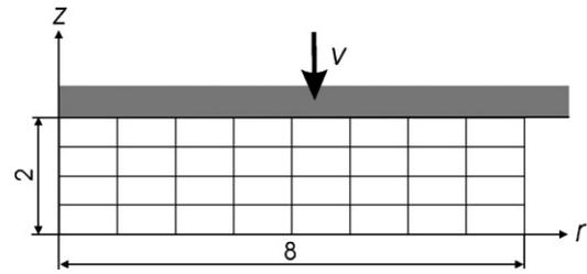
Fig. 3. Geometry and finite element discretization of specimen.
