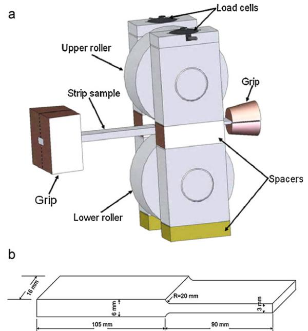
Fig. 1. (a) Schematic illustration of mini two-high rolling mill and (b) schematic illustration of strip sample.
