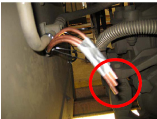
Fig. 3. Two sampling points, brake pad sampling point (right) and global sampling point (left).
