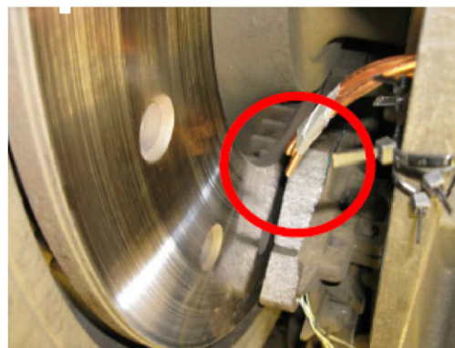
Fig. 3. Two sampling points, brake pad sampling point (right) and global sampling point (left).
