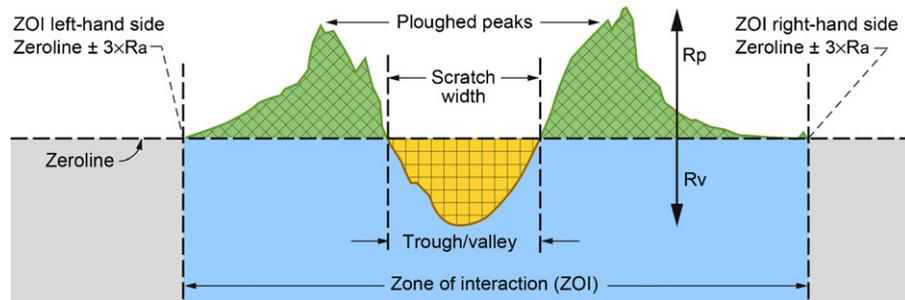
**Fig. 1.** Example of boundary conditions for Zone of Interaction at  $\pm 3 \times$  surface roughness ( $R_a$ ) showing negative and positive displacements.
