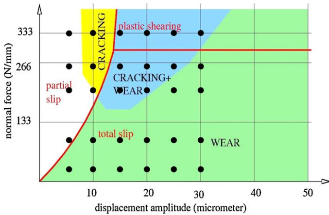
**Fig. 1.** Material response fretting map as determined by [20]. The loading conditions of the computations performed in our study are indicated by black points in the diagram.
