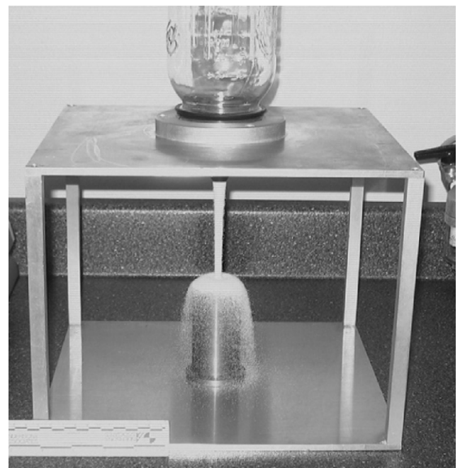
Fig. 2. Uncompacted aggregate void measurement equipment.
