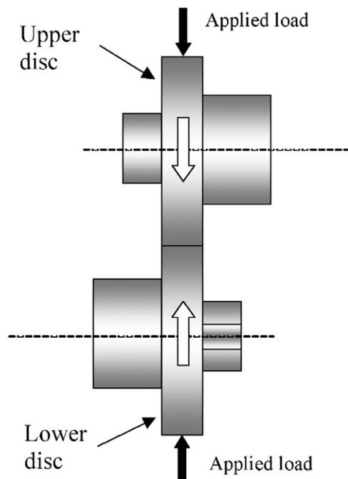
**Fig. 1.** Schematic representation of the testing rig.
