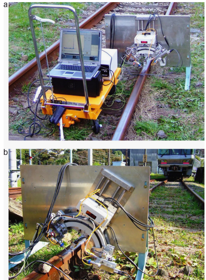
Fig. 1. Appearance of the portable XRDF system installed on the rail, performing analysis for (a) rail top in tangent track and (b) gauge corner of the high rail in curved track.
