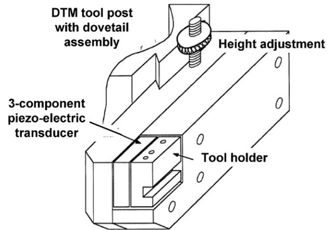
Fig. 2. Diamond tool post incorporating 3-axis piezoelectric load cell (reprinted from [9]).
