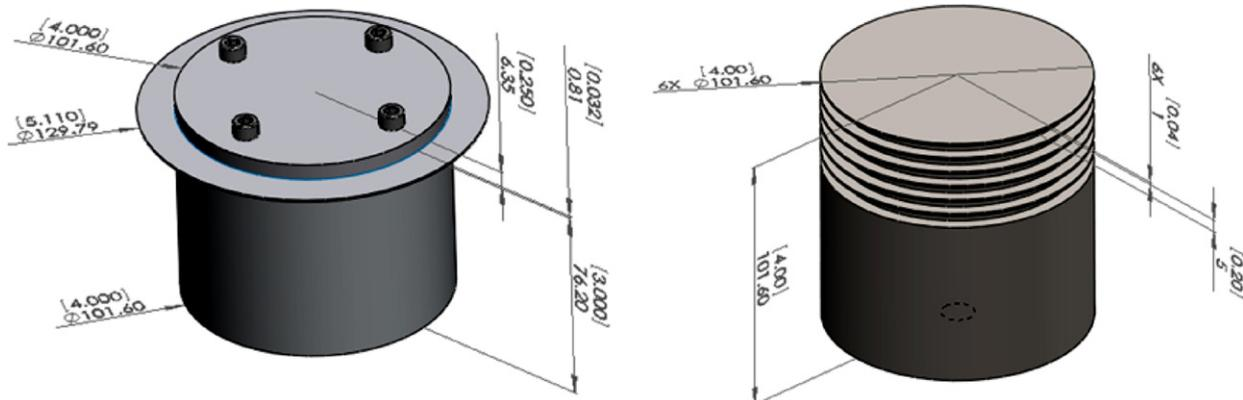
Fig. 1. (Left) holder for replaceable Al6061 disks. (Right) fins created directly in 1215 steel material.
