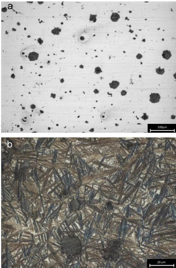
Fig. 1. ADI microstructure. (a) Un-etched condition; (b) after etching with 2% Nital.
