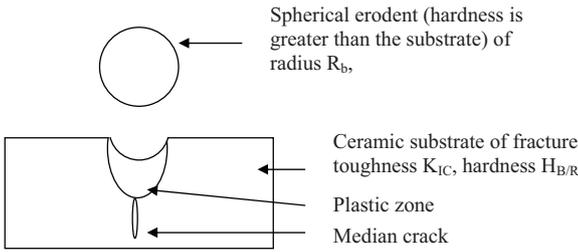
Fig. 2. Schematic diagram of an erosion event by a spherical indenter on a brittle substrate surface causing the formation of median cracks in the surface.
