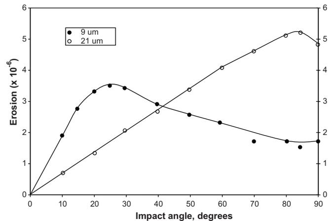
Fig. 7. Dependence of erosion rate on impact angle for soda lime glass eroded by 9 μm and 21 μm SiC particles at 136 m s<sup>-1</sup> [8].
