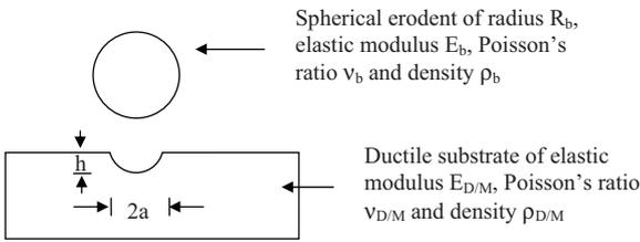
Fig. 1. Schematic diagram of an erosion event by a spherical indenter on a ductile surface.
