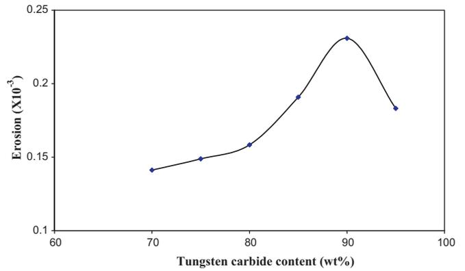
Fig. 5. Erosion rate versus WC content for a WC–Co cermet, following impact by a slurry of 100 μm silicon carbide particles at 40 m s<sup>-1</sup> and at impact angles of 90° [7] (threshold velocity for erosion of Co is 0.21 m s<sup>-1</sup>, and WC is 2652 m s<sup>-1</sup>, according to Eqs. (9) and (13), respectively).
