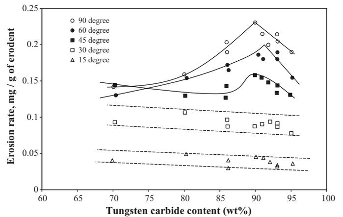
Fig. 6. Erosion rate as a function of WC content for a number of impact angles using 100 μm SiC particles [7].
