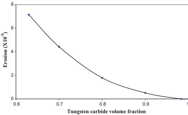
Fig. 4. Erosion rate versus volume fraction of WC for a WC–Co cermet, following impact by a slurry of 10 μm silica particles in oil at 133 m s<sup>-1</sup> and impact angles of 90° [6] (threshold velocity for erosion of Co is 0.21 m s<sup>-1</sup>, and WC is 2651.6 m s<sup>-1</sup>, according Eqs. (9) and (13), respectively).
