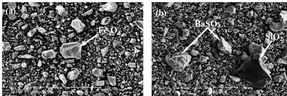
Fig. 2. SEM images of particle morphology of barite and hematite weighting agent.
