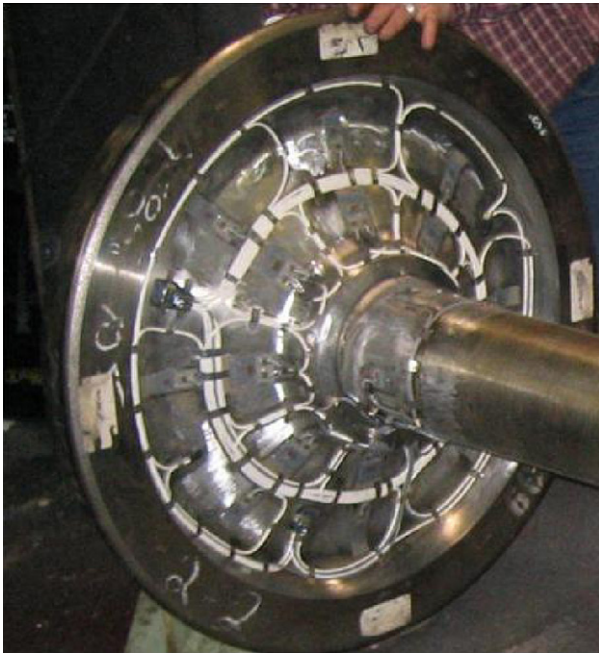
Fig. 1. Strain gauges placed on both sides of the wheel plate are used to measure strains which are then converted into vertical, lateral and longitudinal forces at the wheel/rail contact. A protective coating is applied over the gauges prior to deployment.
