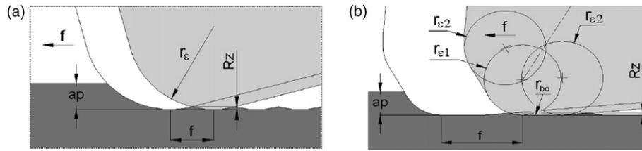
Fig. 1. Comparison of inserts with conventional geometry: (a) and wiper shape; (b) symbols:  $f$  feed;  $a_p$  depth of cut;  $r_e$  radius of the tool corner;  $r_{e1}$  and  $r_{e2}$  radii of wiper curvature;  $r_{bo}$  radius of smoothing part;  $R_z$  valley-to-peak height.
