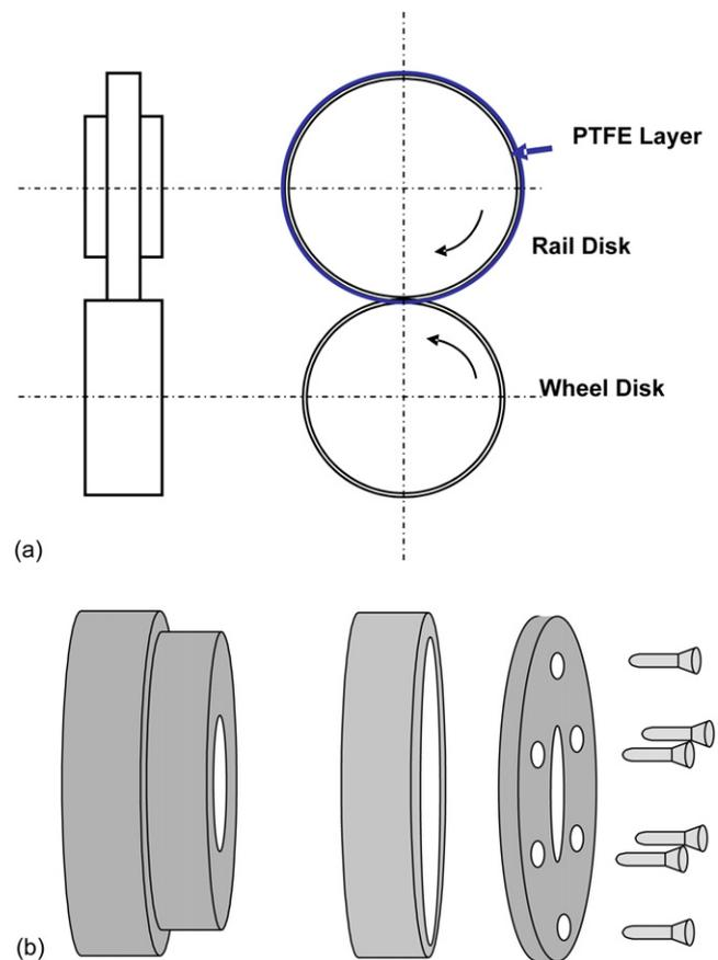
Fig. 1. (a) A disk-on-disk Amsler test machine with two cylindrical disk assemblies running against each other and (b) various parts making up the disk assembly.
