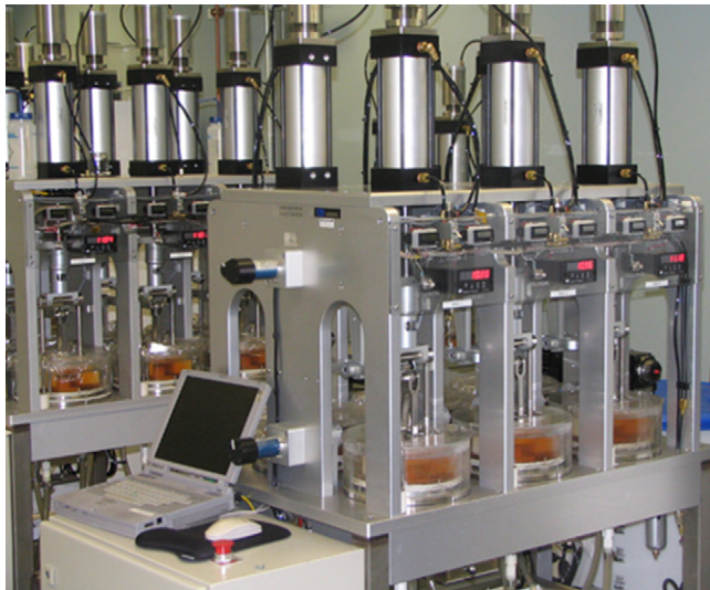
Fig. 1. Laveen spine wear simulator.
