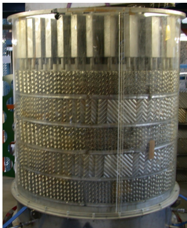
Fig. 1 – Photograph of a short packed bed, consisting of Montz-Pak B1-250, as employed in the present study.
