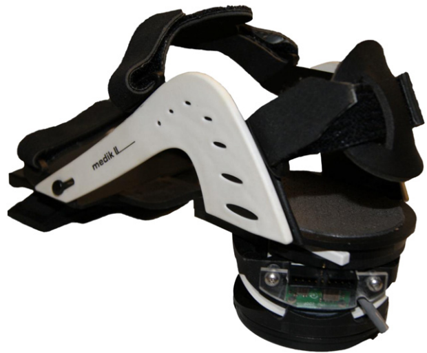
Fig. 1. Illustration of the Myolux Techno™ device. This ankle rehabilitation device has been designed to produce specific ankle inversion in weight bearing conditions. Such an inversion movement can be controlled only by means of ankle evtor muscles eccentric recruitment.
