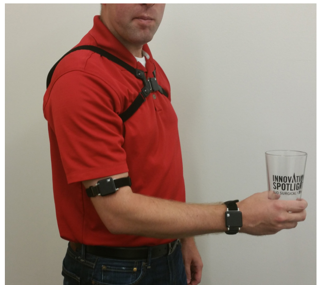
Fig. 1. Placement of inertial measurement units on subject's manubrium and upper arm.
