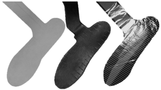
Fig. 1. Test insoles from the three systems: Pedar, Medilogic and Tekscan (left to right).
