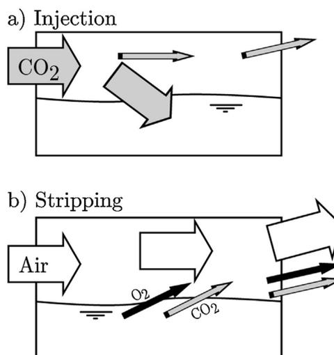
Fig. 1 – Diagram of the carbon dioxide punctual dissolution phase (a) and continuous air stripping phase (b).
