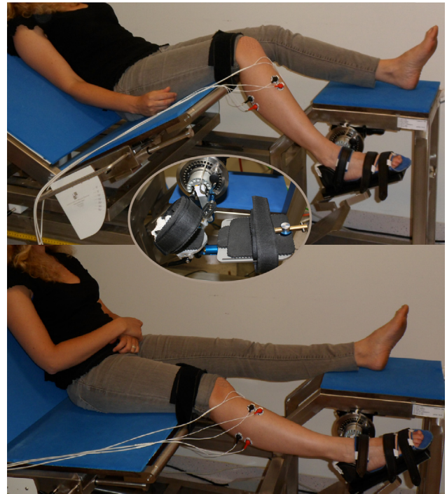
Fig. 1. Measurement set-up with 70^\circ (A) and 20^\circ (B) knee flexion. The rigid footplate is shown in both subfigures, the adjustable footplate is shown in the inset. The broad seating area enabled measurement of either the right or the left foot.
