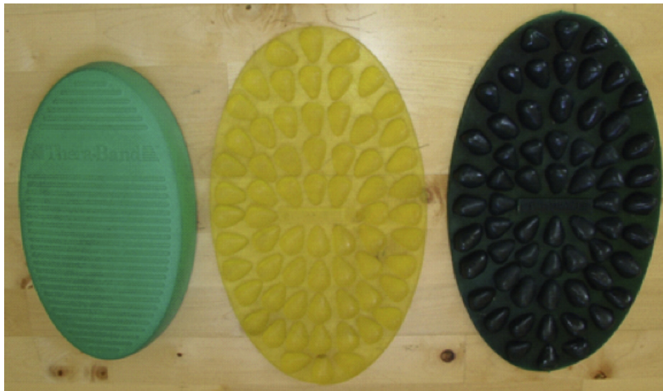
Fig. 1. Photograph of the experimental conditions. From left to right: balance pad (green), soft cobblestone mat (yellow), hard cobblestone mat (black). (For interpretation of the references to color in this figure legend, the reader is referred to the web version of the article.)
