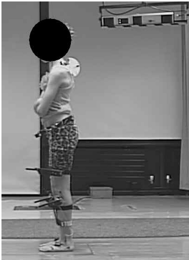
Fig. 1. The Codamotion lower limb marker set and Central Remedial Clinic (CRC) Trunk Model.
