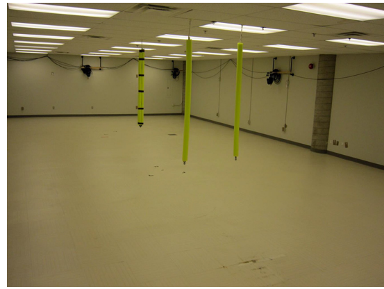
Fig. 1. Setup of the experiment. The obstacles consisted of Styrofoam cylinders which were hung from the ceiling. Obstacle 1 consisted of two obstacles representing a door frame placed 1m30 after the starting point. Obstacle 2 consisted of a foam cylinder placed in the middle of the path, approximately 4m30 through the path.
