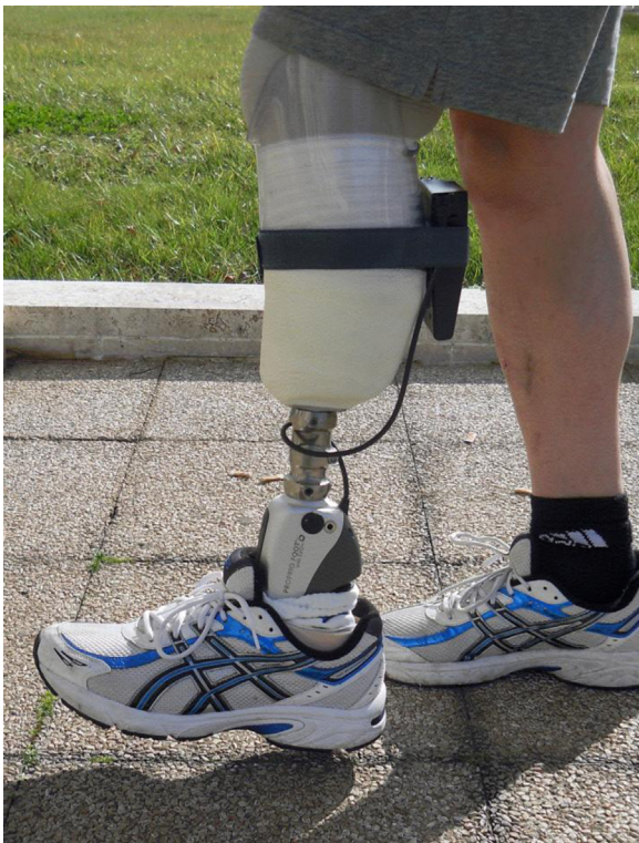
Fig. 1. The Proprio-Foot ® ; during the swing phase it automatically lifts the toe to reduce the risk of trips. Note the battery on the rear side of the socket and the Seal In X5 ® liner under the test socket.
